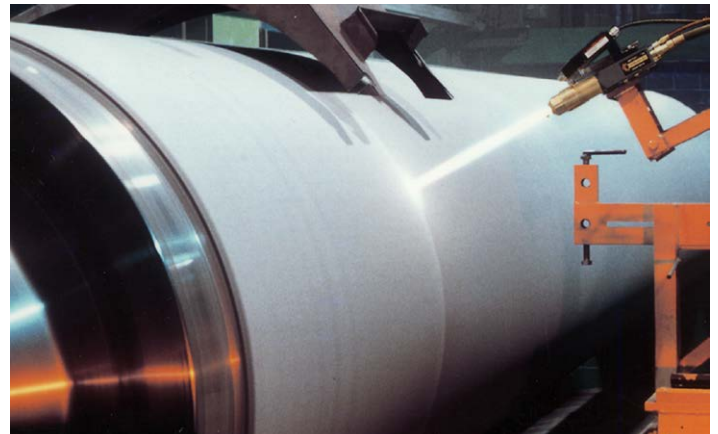
Figure 22 – HVOF coating of a sink roll
