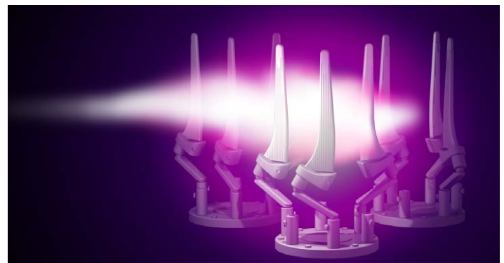
Figure 6b – Controlled atmosphere plasma spraying
