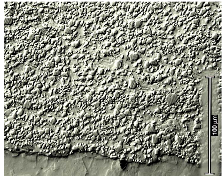
Figure 11 – HVOF spray coating of WC 12(CoCr)
