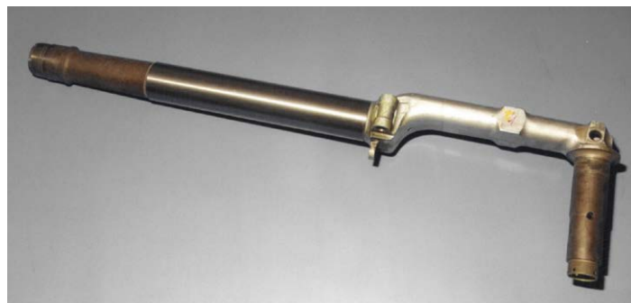
Figure 14 – Nose gear of an F5 Tiger with a WC/CoCr coating
