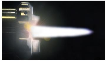
The Oerlikon Metco TriplexPro-210 plasma spray gun with high enthalpy flame.
