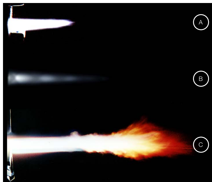
Figure 3. The versatility of the TriplexPro-210 Plasma Spray Gun is demonstrated by these very different plasma jets. A) Standard jet with 9 mm nozzle, B) High velocity jet [ > \text{mach } 1 ], C) High enthalpy jet.
